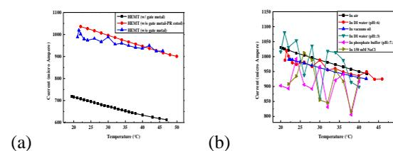
Figure 2. (a) The current of HEMTs with different sensing surface at different temperature in deionized water solution (pH=6). (b) The current of HEMTs without gate metal at different air temperature and in different solutions with different temperature.
