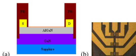
Figure 1. (a) Schematic of the AlGaIn/GaN HEMTs. (b) The top-view of the AlGaIn/GaN HEMTs.
