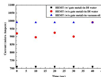
Figure 3. The stability of HEMTs with gate metal and without gate metal, respectively.
