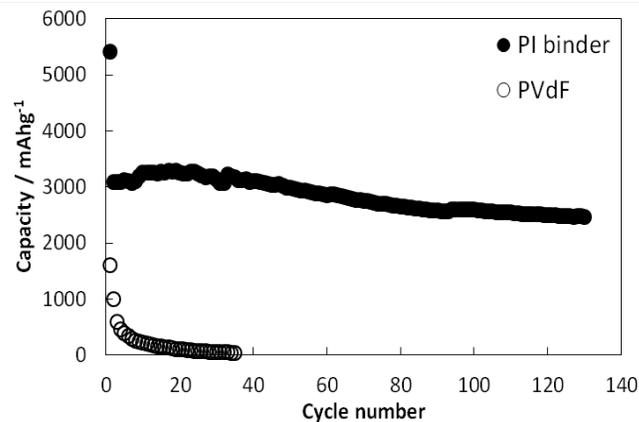
Fig.1 Cycle performance of the silicon negative electrode with PI binder or PVdF charged and discharged at C/20 rate with cut-off 0-1.5V vs. Li
