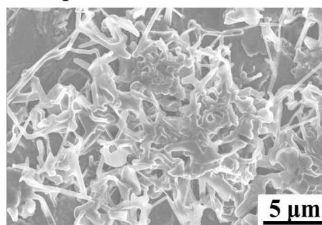
Fig.2 SEM images of silicon negative electrodes and graphite negative electrodes fully charged at C/2 at 0 °C
