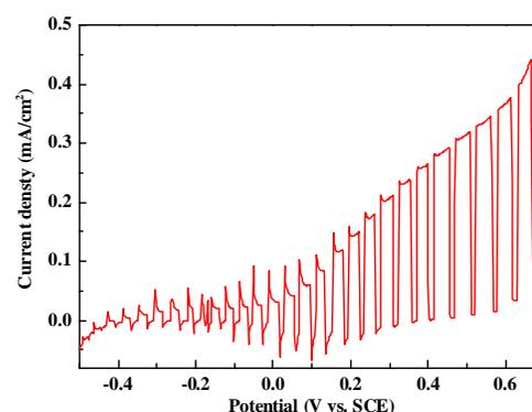
Figure 3. The photocurrent density of hematite annealed at 550°C for 1 h and re-annealed at 750°C for 10 min.
