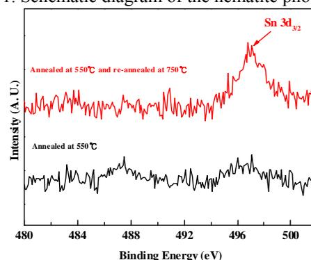
Figure 2. Sn 3d<sub>3/2</sub> XPS spectra of hematite annealed at 550 with and without re-annealed at 750 °C for 10 min.
