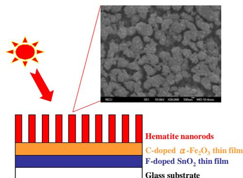
Figure 1. Schematic diagram of the hematite photo anode.
