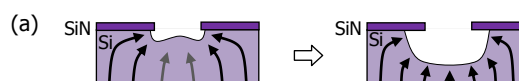
Figure 2. Simplified mechanism of etch form transformation convex-concave during anodization process as effect of current distribution; arrows represent current flow, darker arrows indicate stronger flow.
