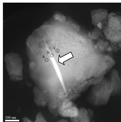
Fig. 2 HAADF-STEM image of 0.98\text{LiMn}_2\text{O}_4-0.02\text{Zn}_2\text{SnO}_4 . Arrows point "Nano Inclusions".
