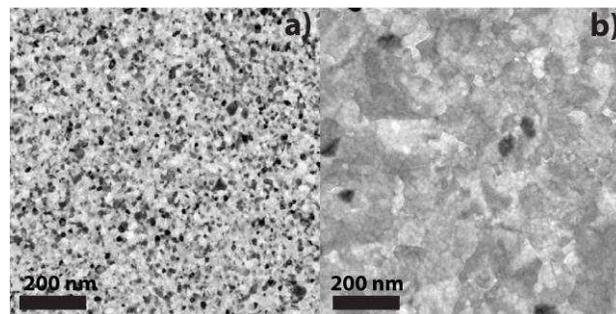
**Fig. 3** Bright-field TEM image of a 15 nm Pt film deposited by plasma-assisted ALD (a). HAADF STEM image of an STO ( $[\text{Sr}]/([\text{Sr}]+[\text{Ti}]) = 0.54$ )/Pt stack after RTA at 600 °C for 1 min.
