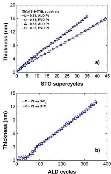
**Fig. 1** STO film thickness evolution of STO on Pt (deposited by ALD and PVD) as measured by in-situ SE (a) and Pt film thickness evolution on STO and SiO<sub>2</sub> (b).
