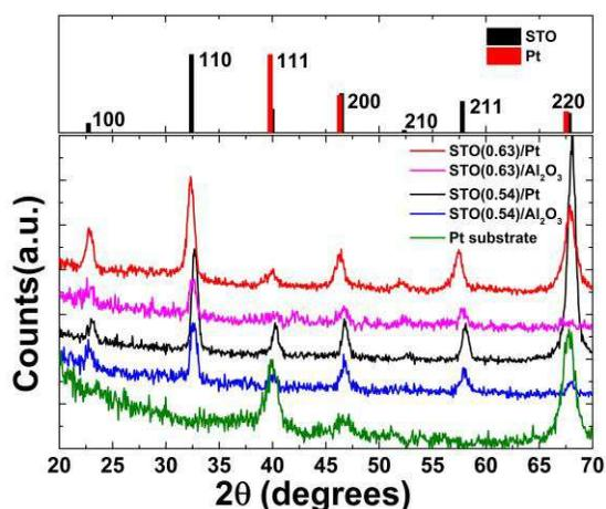
**Fig. 2** GI-XRD patterns of STO films with  $[\text{Sr}]/([\text{Sr}]+[\text{Ti}]) = 0.54$  and  $0.63$  grown on Pt and on Al<sub>2</sub>O<sub>3</sub> after RTA at 600 °C for 1 min. The GI-XRD of the Pt substrate is included as a reference.
