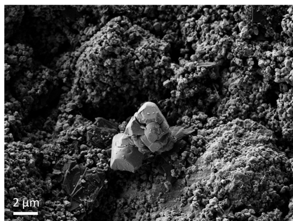
Fig. 1: SEM image of a manganese oxide particle on a LTO anode.
