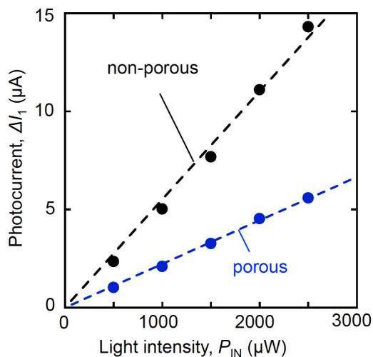
**Fig. 3** Comparison of photocurrents between non-porous and porous devices plotted as function of  $P_{\text{IN}}$ .
