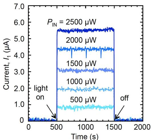
**Fig. 2** Current response properties of porous PC device based on incident light at various power levels,  $P_{\text{IN}}$ .
