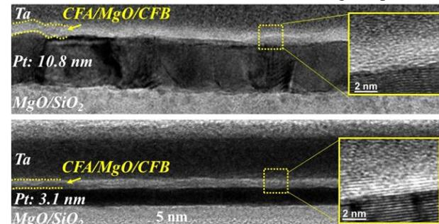
Fig. 4. Cross-sectional HR-TEM Images of p-MTJ stacks at  $T_{ex}=300^\circ\text{C}$ .
