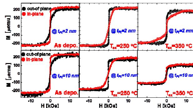
Fig. 1.  $M-H$  curves in out-of plane & in-plane for p-MTJs with  $t_{Pt}=2$  and 10 nm without and with annealing at 250 and 350°C.
