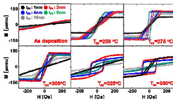
Fig. 2.  $M-H$  curves in out-of-plane direction for p-MTJ stacks without and with annealing at to temperature ranging from 250 to 350°C
