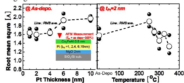
Fig. 3. Surface roughness (RMS) for p-MTJ stack with  $t_{Pt}=1, 2, 4, 6,$  and 10 nm at various annealing temperatures.
