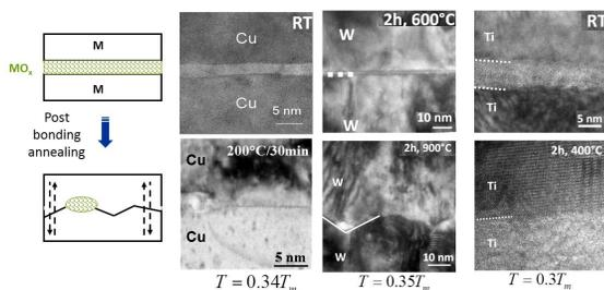
Fig 1 :TEM observation of the metal bonding interface. At room temperature each bonding interface present an thin metal oxide layer. At 0.3T<sub>m</sub> the oxide layer is instable and is dissolved. The electrical behavior is perfect.
