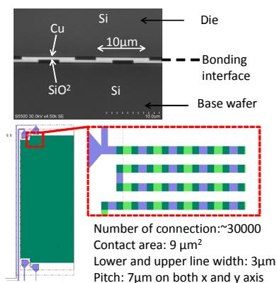
Fig 3: SEM observation of a copper daisy chain with a 7µm pitch.
