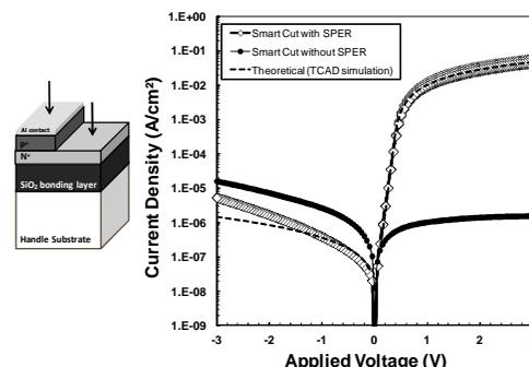
Fig 2. I(V) diode characteristics after Smart Cut<sup>TM</sup> layer transfer
