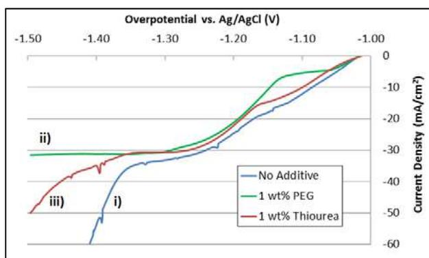
**Figure 1.** Polarization curves on a zinc-coated wire electrode in 0.1 M ZnCl<sub>2</sub> containing: i.) No additive, ii.) 1 wt% PEG, iii.) 1 wt% thiourea.
