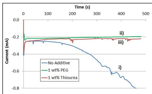
**Figure 2.** Potentiostatic plating at an overpotential = -1.25 V vs. Ag/AgCl on PVC-coated wire in 0.1 M ZnCl<sub>2</sub> containing: i.) No additive, ii.) 1 wt% PEG, iii.) 1 wt% thiourea.
