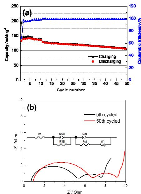
**Fig. 2** (a) Capacity fading of a full cell using a Si-graphene negative electrode and LiMO<sub>2</sub> positive electrode at C-rates of C/15 in 1<sup>st</sup> ~ 5<sup>th</sup>, C/5 in 5<sup>th</sup> ~ 10<sup>th</sup>, and C/2 in 10<sup>th</sup> ~ 50<sup>th</sup>. (b) EIS curves of the full cell after the 5<sup>th</sup> and 50<sup>th</sup> cycle.
