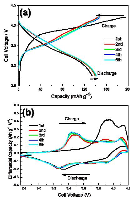
**Fig. 1** Charge/discharge curves (a) and differential capacity curves (b) of full cells employing Si-graphene negative electrode and LiMO<sub>2</sub> positive electrode for the first 5 cycles at C/15 between 2.75 and 4.2 V.
