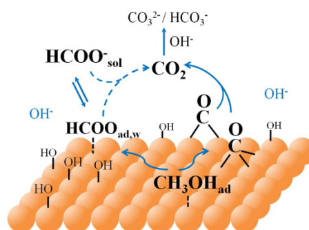
Scheme 1. Schematic diagram for methanol dissociation and electro-oxidation at Pd electrode in alkaline media [3].
