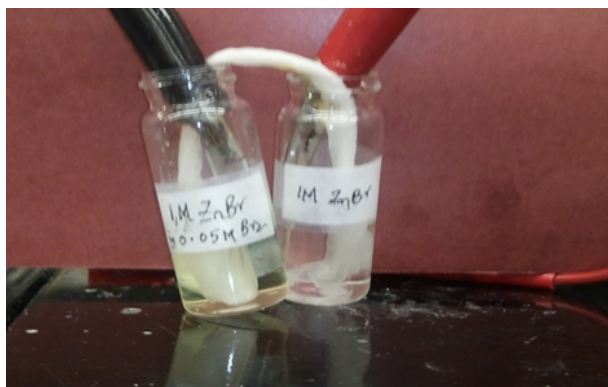
Figure 1. Experimental set up of the Zn-Br flow battery system for preliminary data.
