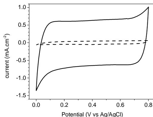
Fig. 2: voltamogram at 5 mV/s of a 200 nm MnO<sub>2</sub> coated 40 μm depth pillars electrode (line) in an aqueous electrolyte of 0.5M Na<sub>2</sub>SO<sub>4</sub> and comparison with a 100 nm MnO<sub>2</sub> coated flat electrode (dash)
