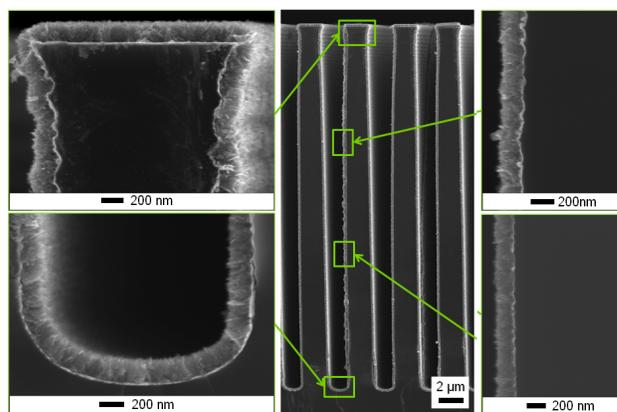
Fig. 1: SEM cross section view of microwalls coated by a conformal 200 nm pulsed electrodeposited MnO<sub>2</sub> layer on an ALD-deposited 30 nm platinum current collector.
