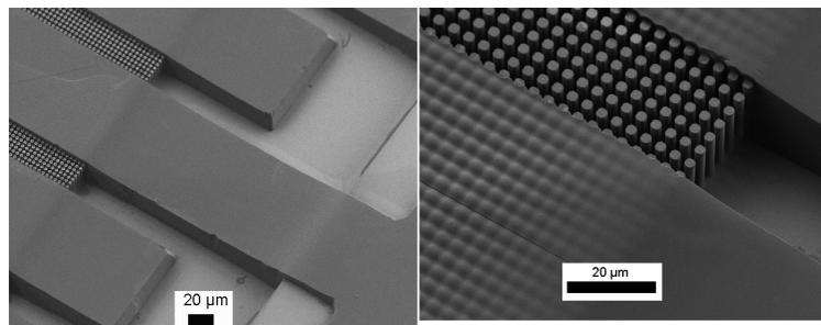
Fig. 3: SEM views of the photolithography step before etching of the platinum current collector
