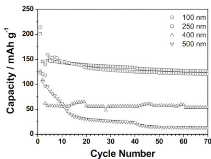
Fig.1 The cycling performance of 3d TiO<sub>2</sub> nanofiber electrodes with different diameters
