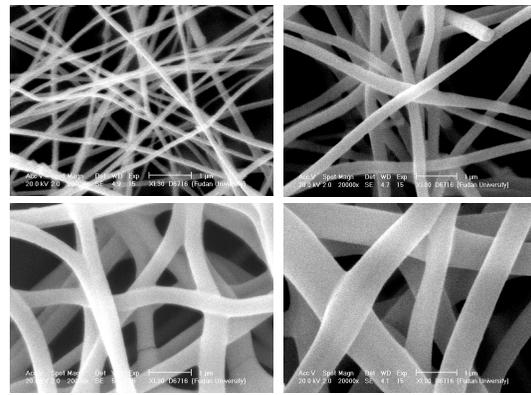
Fig.3 The SEM image of TiO<sub>2</sub> nanofibers with different diameters(a)100nm;(b)250nm;(c)400nm;(d)500nm
