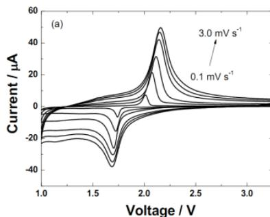
Fig.2 CV measurements for Li/TiO<sub>2</sub> nanofiber cell with the diameter around 250 nm
