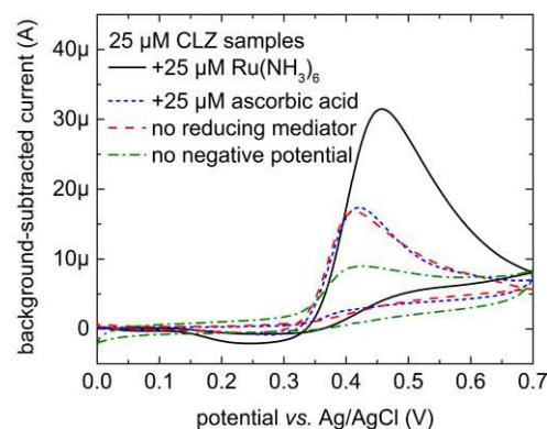
**Figure 3.** Cyclic voltammetry using phosphate buffer spiked with CLZ and either Ru(NH<sub>3</sub>)<sub>6</sub>, ascorbic acid, or neither. For the latter, a cycle limited to positive potentials is also shown.
