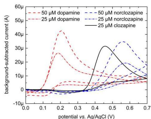
**Figure 2.** Cyclic voltammetry using phosphate buffer spiked with Ru(NH<sub>3</sub>)<sub>6</sub> and either CLZ, norclozapine, or dopamine.
