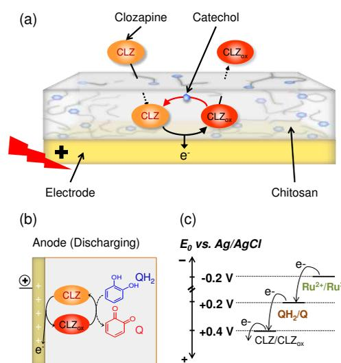
**Figure 1.** CLZ as an oxidizing mediator in the catechol-modified chitosan system. (a) Schematic of the system with the diffusing CLZ. (b) Continuous oxidation of CLZ in the presence of catechol (Q) reduction. (c) Standard reduction potentials and electron transfers in the system.
