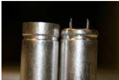
Can and finished nominally 100 F sealed electrochemical capacitor
