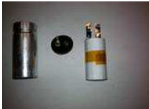
Can, header, and spiral wound electrode-separator bobbin
