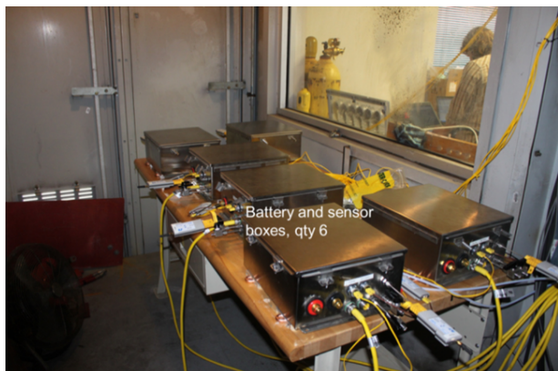
Figure 1 Testing boxes for atmospheric and temperature control of battery cells.
