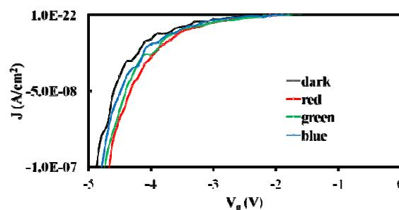
Figure 2.  $J$ - $V$  curves of the  $\text{WO}_x$  sample under the  $-V_g$  range.
