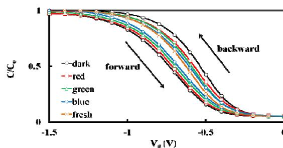
Figure 1.  $C$ - $V$  hysteresis of the  $\text{WO}_x$  sample from  $-5 \text{ V}$  to  $+5 \text{ V}$  to  $-5 \text{ V}$  at 1 MHz under different light illuminations.
