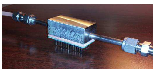
Fig. 2: Flow through gas sensor testing chamber design
