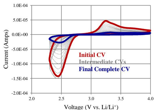
Figure 2. Cyclic voltammograms of polycrystalline Au disk from 2.3 to 4 V vs. Li. Scan rate is 100 mV/sec.
