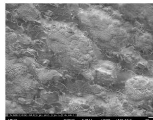
Fig. 2. Microfractograph of UD-165 after a fatigue test at  $\Delta K=153.5 \text{ MPa}\sqrt{\text{cm}}$  in  $\text{NaCl}/\text{NaHCO}_3/\text{Na}_2\text{CO}_3/p_{\text{H}_2\text{S}} = 0.83 \text{ kPa}$  at 20°C, pH=7.
