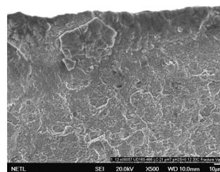
Fig. 1. Microfractograph of UD-165 after a fatigue test at  $\Delta K=219.8 \text{ MPa}\sqrt{\text{cm}}$  in  $\text{NaCl}/\text{NaHCO}_3/\text{Na}_2\text{CO}_3/p_{\text{H}_2\text{S}} = 0.83 \text{ kPa}$  at 20°C, pH=7.
