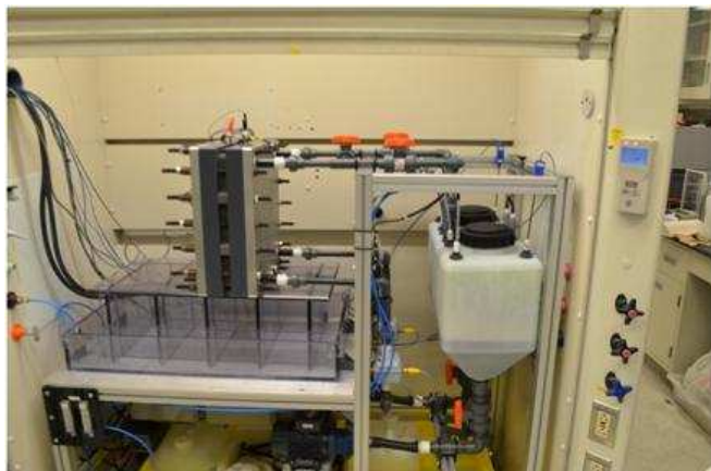
Figure 1. PNNL Redox Flow Battery Test Stand.
