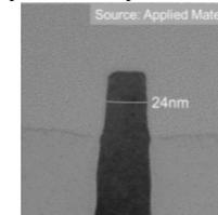
Figure 5d. Wide fin of 24nm CD with room temperature SDE implant was single crystalline after spike anneal
