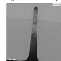
Figure 7a. Fin after halo implant at room temperature
