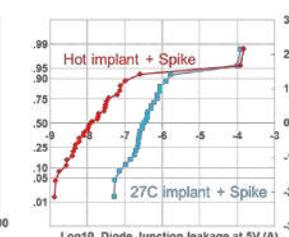
Figure 4. Junction leakage comparison hot vs. room temperature implant
