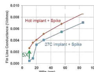
Figure 3. Fin conductance vs. fin width comparison hot vs. room temperature implant
