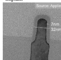
Figure 5b. Wide fin of 32nm CD with 7nm amorphous outerlayer post room temperature SDE implant
