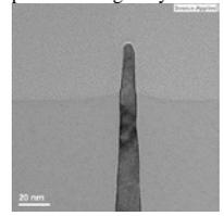
Figure 7b. Fin after halo implant at room and split anneal
