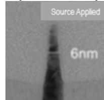
Figure 5c. Narrow fin of 6nm CD with room temperature SDE implant was polycrystalline after spike anneal
