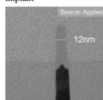
Figure 5a. Narrow fin of 12nm CD completely amorphized by room temperature As SDE implant
