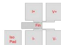
Figure 2. Fin resistor layout
