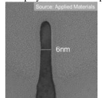
Figure 6. Hot SDE implant produces single crystalline 6nm fin
