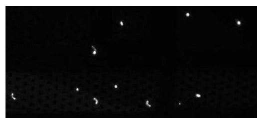
Figure 3: Biotinylated fluospheres (1 \mu\text{m} diameter) were flown (linear velocity 24 cm/min) into a channel (150 \mu\text{m} wide, 6.5 \mu\text{m} tall) and captured by rotating streptavidin coated M-280 beads (2.8 \mu\text{m} diameter). In the image, M-280 beads were rotating at 2500 rpm (linear velocity 2.3 cm/min). Bound fluospheres show up as streaklines due to the exposure time needed to detect fluorescence.
