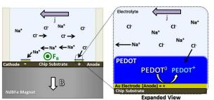
Right shows distant view of the PEDOT film, oppositely biased electrodes, magnet location, and expected fluid flow. When a potential is applied to the electrodes, anions must come in and out of the PEDOT film to compensate for the change in charge. Left shows expanded view of the PEDOT film on the anode. As PEDOT is oxidized, anions (Cl-) must come into the film.
