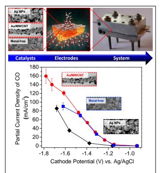
**Figure. 1.** Top: Overview of our recent efforts to understand and improve catalysts, electrode structure, and operating conditions. **Bottom:** Results of the electrochemical reduction of  $CO_2$  to CO using the flow reactor operated with three different high-performance cathode catalysts, *i.e.*, silver nanoparticles (black curve)<sup>[4]</sup>, metal-free catalyst (blue curve), and metal nanoparticles supported on multiwall carbon nanotubes (Au/MWCNT) (red curve).
