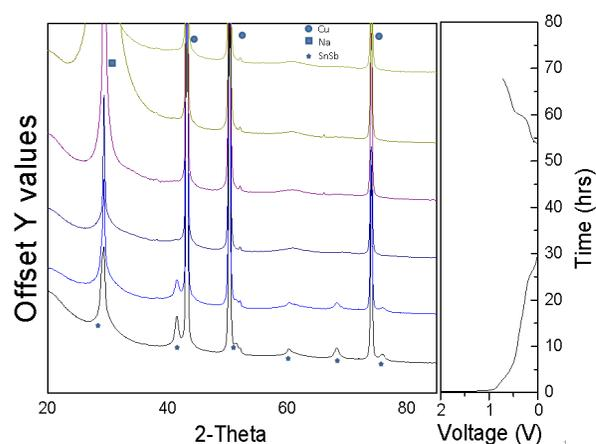
Figure 2. XRD patterns and corresponding voltage profile of the in situ Na/SnSb alloy anode cell.
