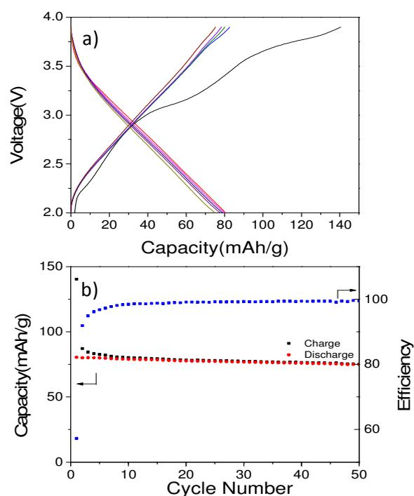
Figure 1: (a) Voltage profiles of SnSb/NaNi<sub>1/3</sub>Mn<sub>1/3</sub>Fe<sub>1/3</sub>O<sub>2</sub> between 2-3.9V, from right to left 1<sup>st</sup> cycle, 5<sup>th</sup> cycle, 10<sup>th</sup> cycle, 20<sup>th</sup> and 50<sup>th</sup> cycle. (b) Cycling performance of SnSb/NaNi<sub>1/3</sub>Mn<sub>1/3</sub>Fe<sub>1/3</sub>O<sub>2</sub> at a current rate 10mA/g based on the active cathode material
