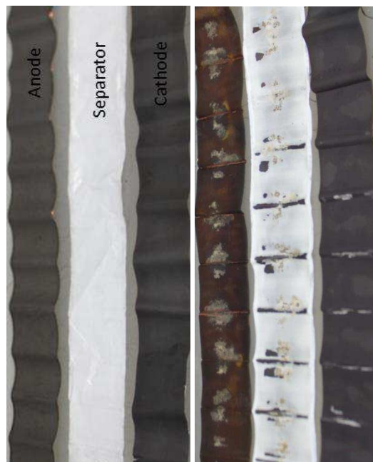
Figure 2. Photographs of a pristine cell (left) and a cell cycled under an initial stack pressure of 0.1 MPa. Spatially non-uniform lithium content in the anode can be seen based on graphite coloration as well as the presence of localized surface films.
