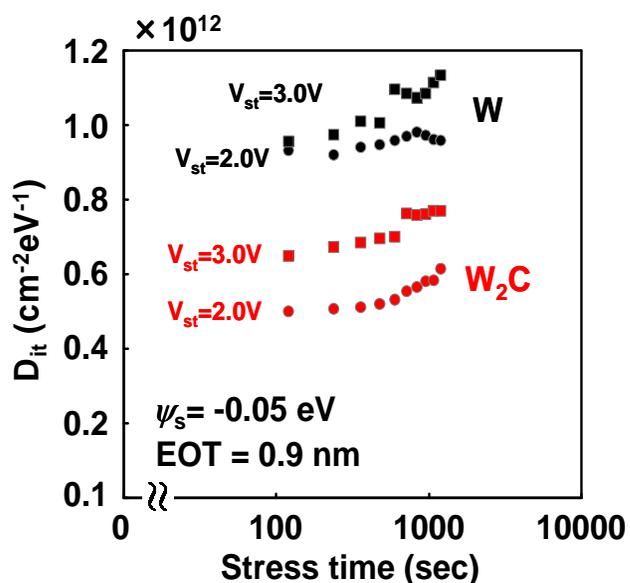
Fig. 3 Interface state density ( $D_{it}$ ) versus stress time plot on different stress bias
