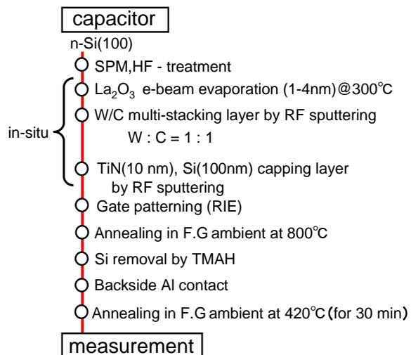
Fig. 1 Device fabrication process
