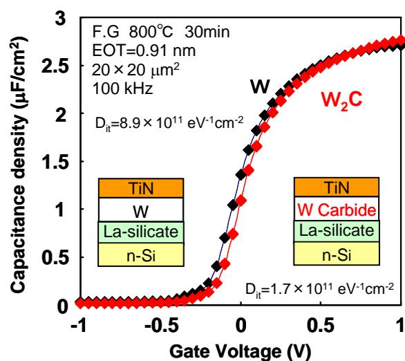
Fig. 2 C-V characteristics of TiN/ $\text{W}_2\text{C}$ /La-silicate/*n*-Si and TiN/W/La-silicate/*n*-Si capacitors
