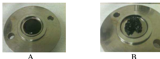
Figure 2. Phase change after addition of CNTs (>1wt%) on neat ILs. A: PMII/CNT 0.2 wt%. B: PMII/MWCNT 1.5 wt%
