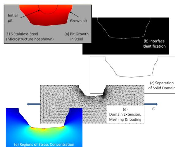
Figure 1. Simulation steps from pitting to mechanical loading.
