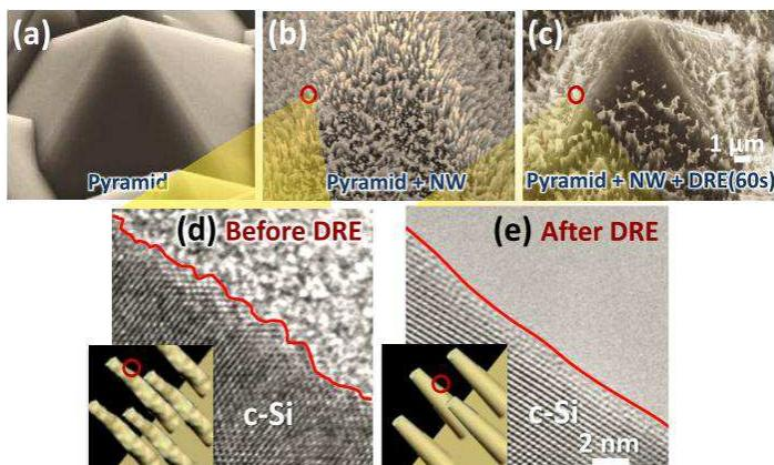
**Figure 1.** (a)-(c) SEM images at various stages for fabricating hierarchical structures with DRE. HRTEM images taken near the edge of the individual NW on hierarchical structures (d) before and (e) after DRE.
