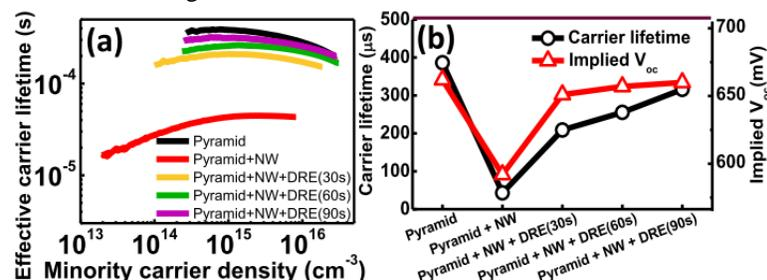
**Figure 3.** (a) Effective carrier lifetime as a function of minority carrier density for the hierarchical structures with different DRE durations compared with micropyramid surfaces. (b) Lifetimes at carrier density of 10<sup>15</sup> cm<sup>-3</sup> and implied  $V_{oc}$  of all structures.
