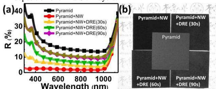
**Figure 2.** (a) Total reflectance of the hierarchical structures with different DRE durations compared with micropyramid surfaces. (b) A photographic image of five structures on 4 \* 4 cm<sup>2</sup> wafers.
