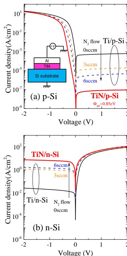
Fig. 1 J-V characteristics of (a) TiN and Ti contacts on n-Si and (b) TiN and Ti contacts on p-Si. Measurement temperature for all samples is RT.
