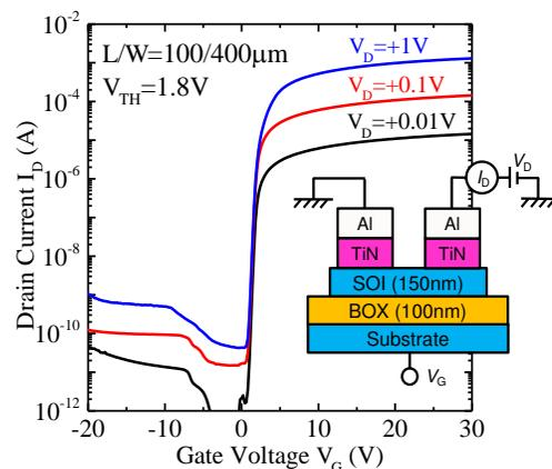
Fig. 2  $I_D$ - $V_G$  characteristic for the fabricated inversion-mode back-gate MOSFET. The cross-sectional schematic image of the MOSFET is also shown as an inset.
