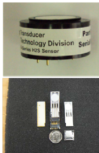
Figure 1. Conventional (top) and prototype printed (bottom) amperometric gas sensors.
