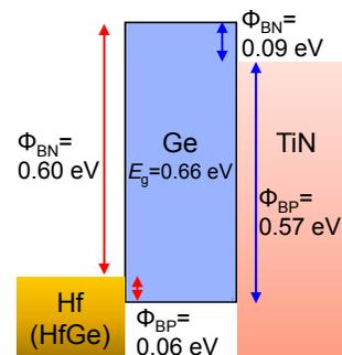
**Fig. 1** Band diagram of HfGe/Ge and TiN/Ge contacts. The HfGe/Ge and TiN/Ge are preferable as low barrier height contacts for hole and electron, respectively.
